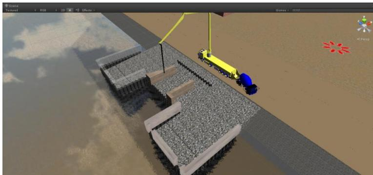
Fig. 6. Casting the retaining walls surrounding inclined level.
