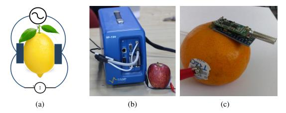
Fig. 7. (a) Bio-impedance measurement schematic. (b) *SP*150 impedance analyzer experimental setup. (c) Portable impedance analyzer.
