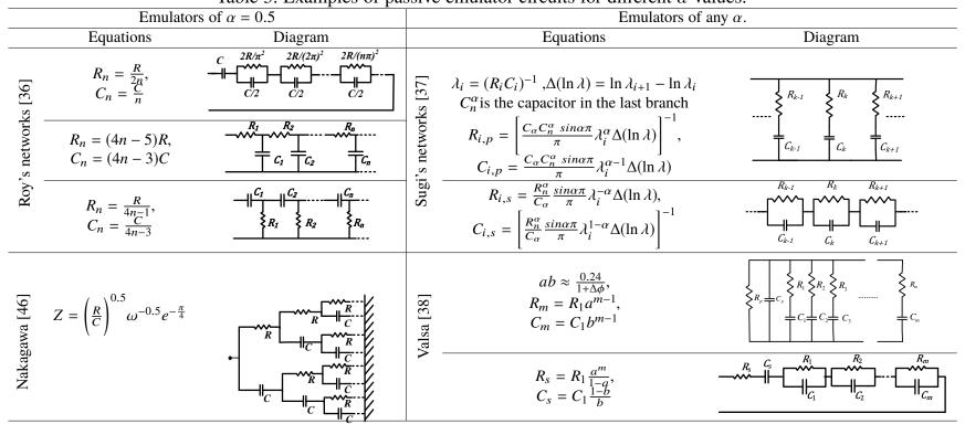
Table 3. Examples of passive emulator circuits for different  $\alpha$  values.
