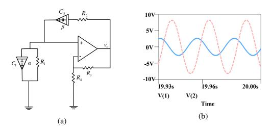
Fig. 5. (a) Wien-bridge oscillator, and (b) Simulation results.
