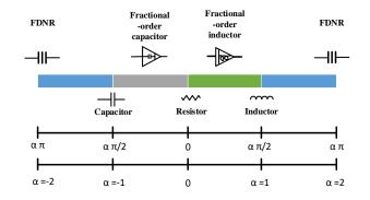
Fig. 3. Conventional elements and their relation to the fractional ones.
