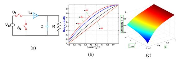
Fig. 8. (a) Buck converter. (b) Gain vs duty cycle. (c) The efficiency.
