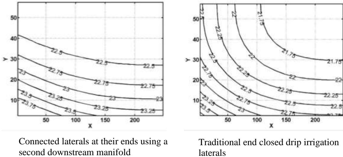
Fig. 8. Isolines of emitter out flow for manifold diameter of 75 mm and lateral diameter of 13 mm.
