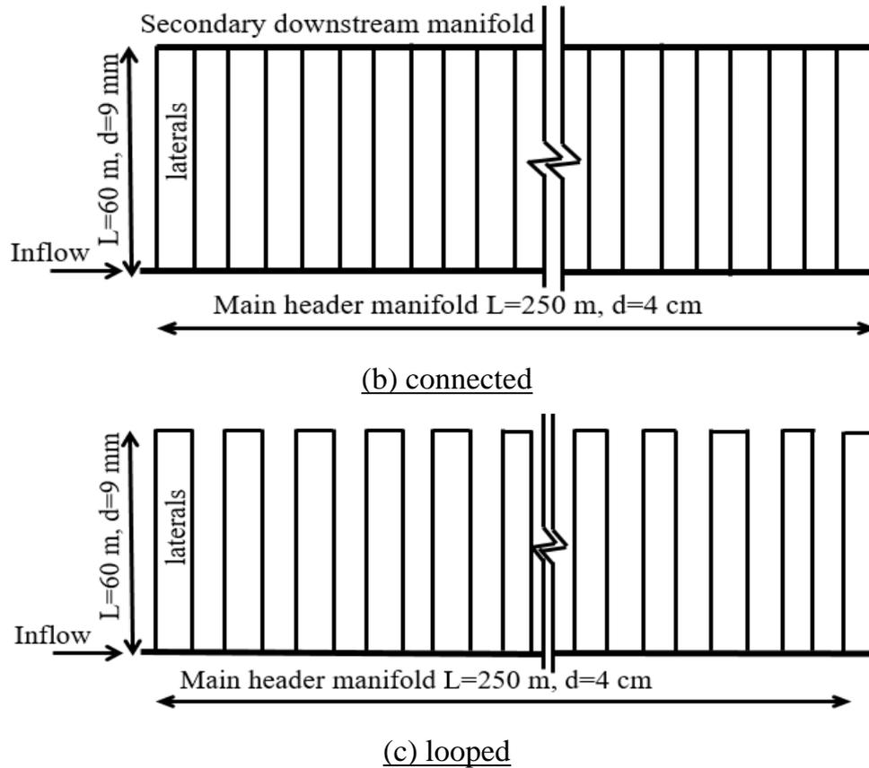
Fig. 1. Layout of the drip irrigation systems for the three lateral alternatives.
