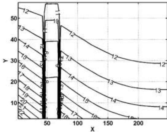
Connected laterals at their ends using a second downstream manifold (clogging of 5 laterals)
