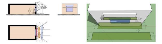
Fig. 5. South orientation model and resulting limiting planes of the sun shading device.
