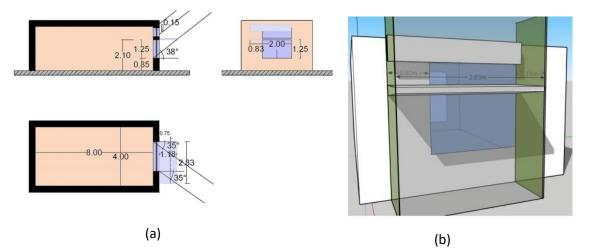
Fig. 3. East orientation model and resulting limiting planes of the sun shading.
