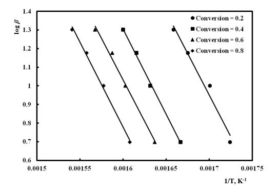
Fig. 4. FWO plots for the pyrolysis of cigarette butts.
