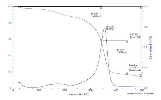
Fig. 1. TG – DTG curves for the pyrolysis of cigarette butts at heating rate =  $10 \text{ K.min}^{-1}$ .
