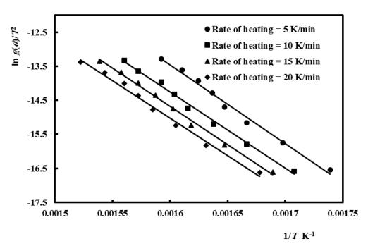
Fig. 5. Coats - Redfern plots for the pyrolysis of cigarette butts.
