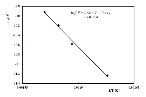
Fig. 3. Kissinger plot for butt fibers pyrolysis.
