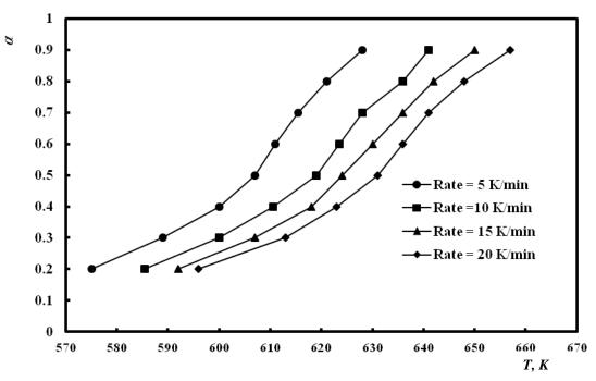
Fig. 2. Effect of heating rate on conversion – temperature curves.
