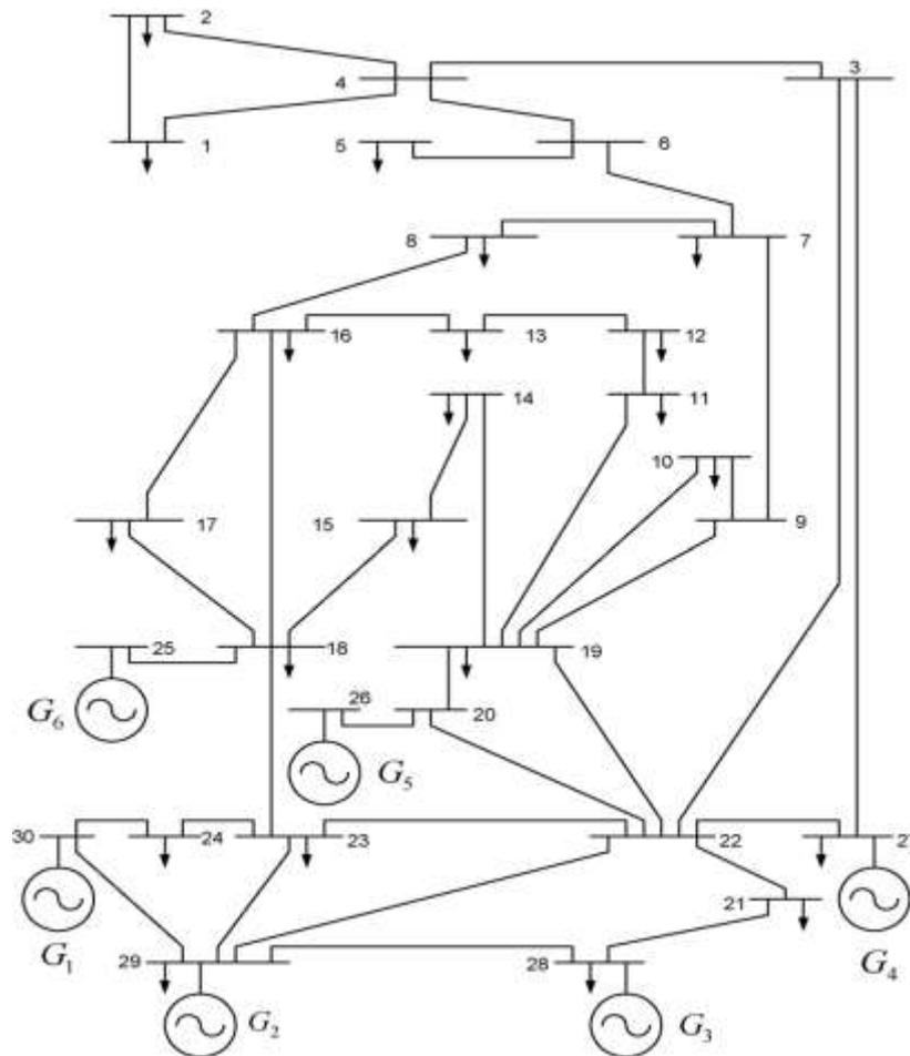
Fig. 2. Single-line diagram of IEEE 30-bus test system [34].
