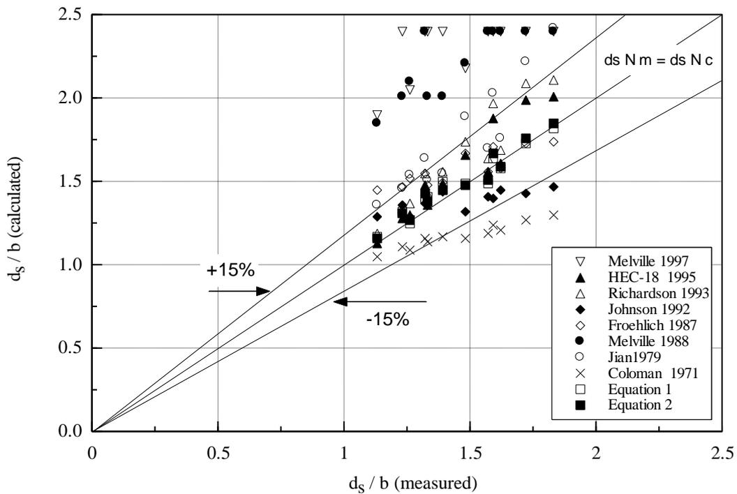
Fig. 3. Comparison between measured and calculated normalized scour hole depth.
