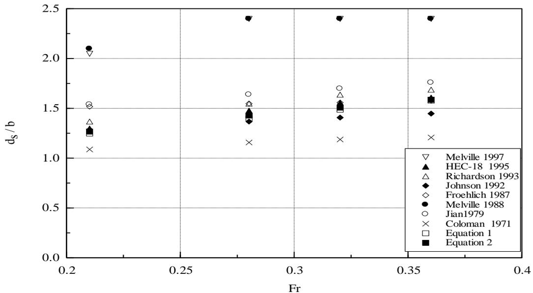
Fig. 2-b. Comparison between calculated normalized scour depth with Froude Number for 10cm pile diameter.
