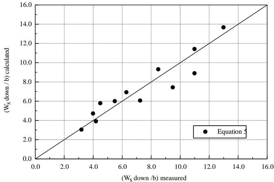
Fig. 6. Comparison between measured and calculated scour hole width downstream of circular pile.
