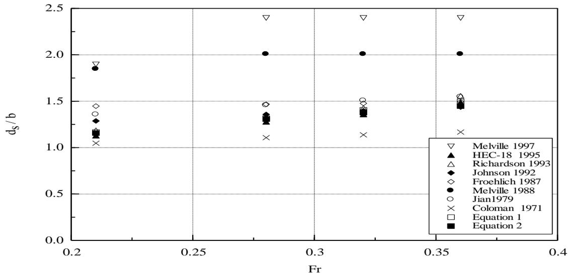
Fig. 2-c. Comparison between calculated normalized scour depth with froude number for 15cm pile diameter.
