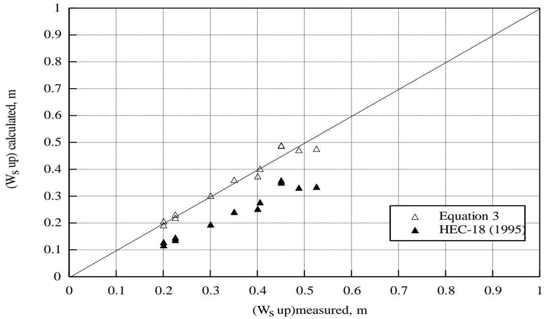
Fig. 4. Comparison between measured and calculated scour hole width upstream of circular pile.
