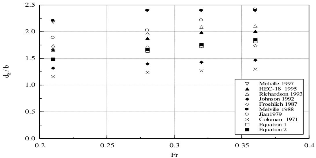
Fig. 2-a. Comparison between calculated normalized scour depth with Froude Number for 5cm pile diameter.
