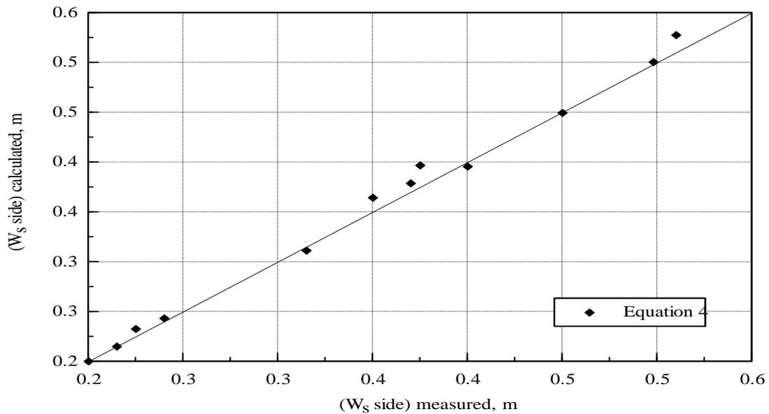
Fig. 5. Comparison between measured and calculated scour hole width at pile's side for circular pile.
