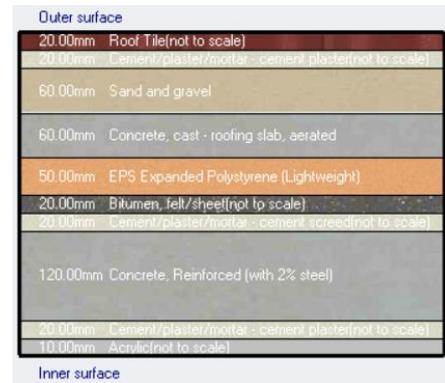
Fig. 9. Roof layers in normal case.
