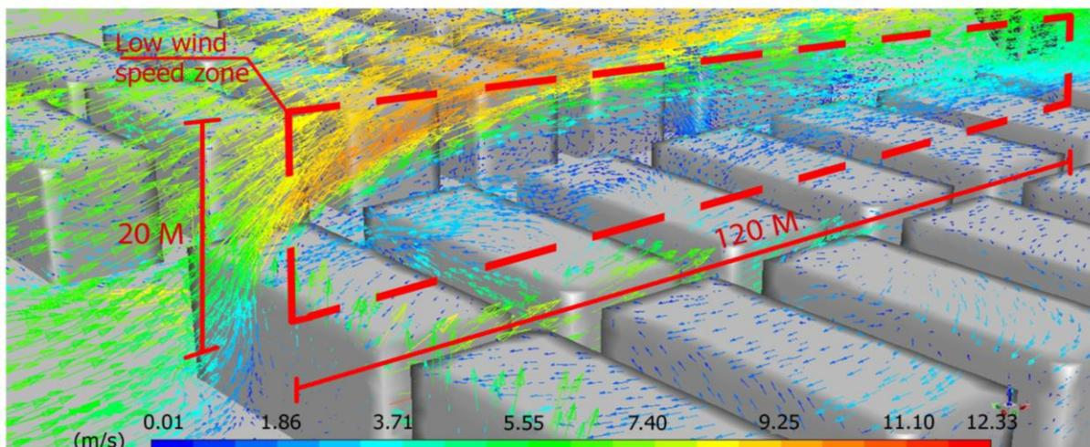
Fig. 9. Low wind speed zone created above buildings in alternatives 1 and 2 by ANSYS Fluent software (version19), inlet wind velocity 7m/s.
