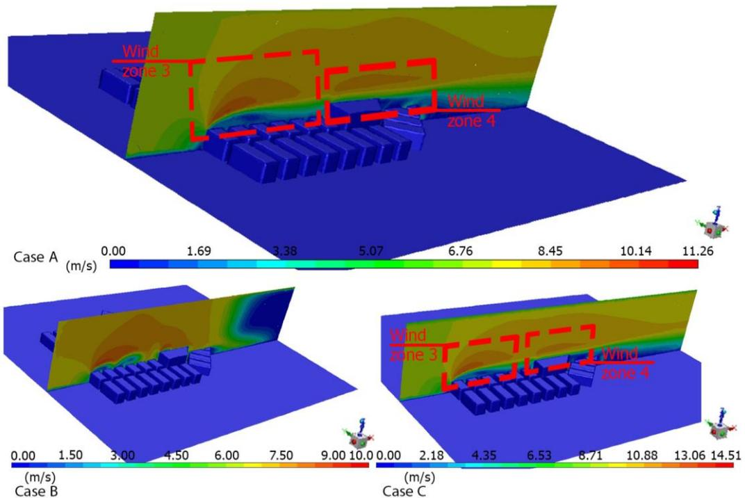
Fig. 8. Alternative 2, wind speed magnitude at section 2 in ANSYS Fluent software (version 19) showing wind zones 3 and 4.
