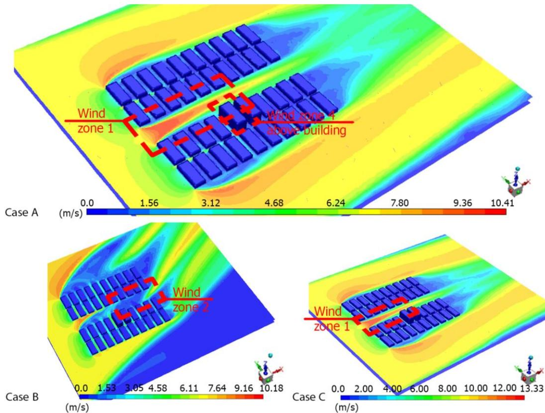
Fig. 5. Alternative 1, wind speed magnitude at height 15 m above street level in ANSYS Fluent software (version19) showing wind zones 1, 2 and 4.
