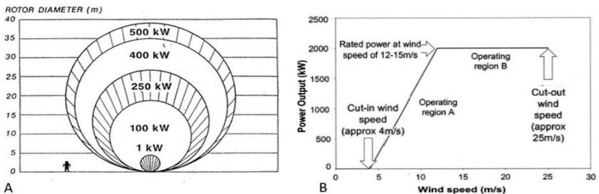
Fig. 2. A) Rotor diameter versus output generated power, B) Wind speed versus generated power output, [21].
