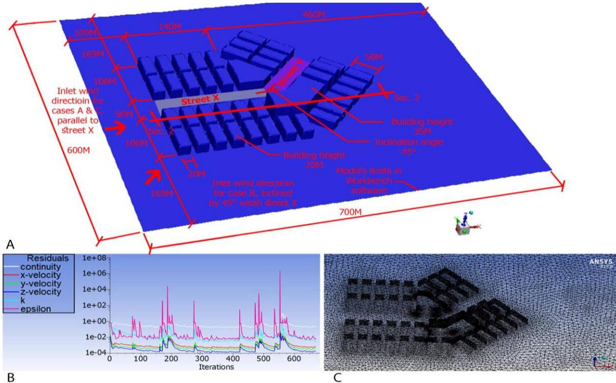
Fig. 4 Alternative 2, A) dimensions and inlet wind directions, B) Residuals by ANSYS Fluent software, C) Mesh by ANSYSWB module software.
