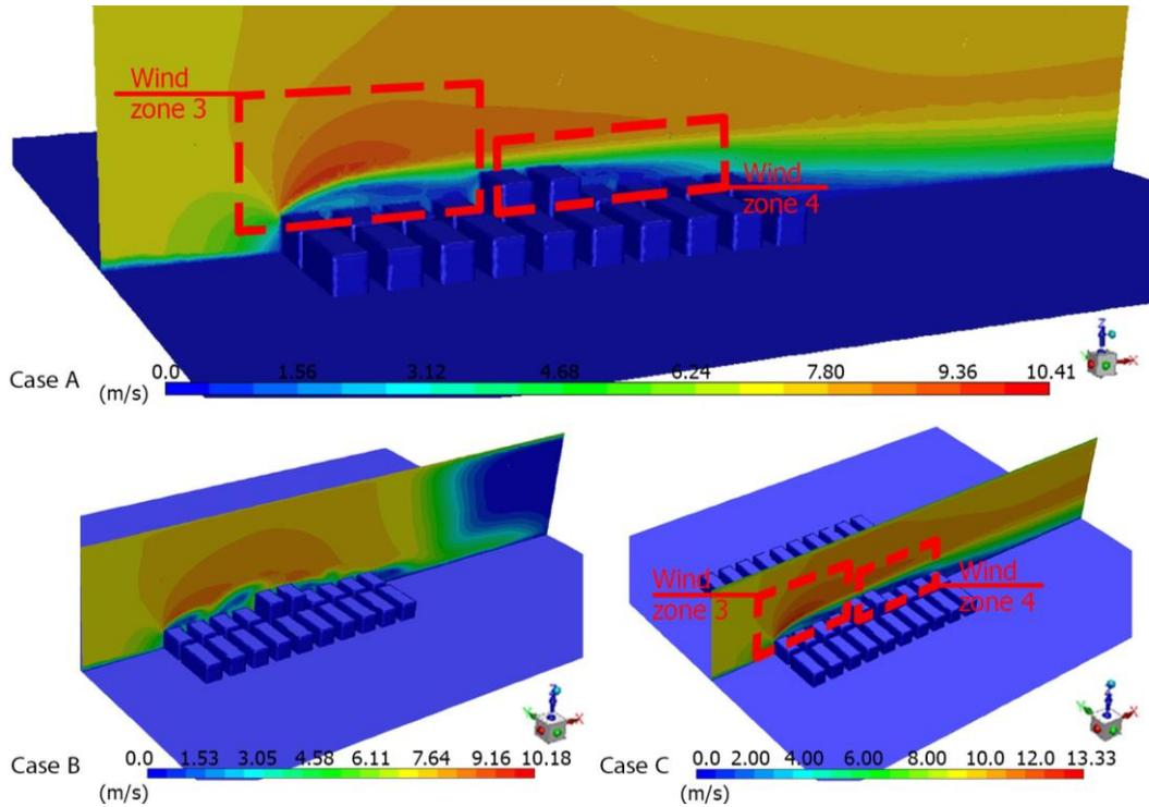
Fig. 7. Alternative 1, wind speed magnitude at section 1 in ANSYS Fluent software (version 19) showing wind zones 3 and 4.
