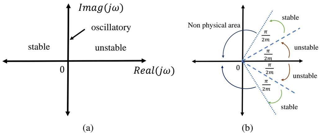
Fig. 4. The stability regions for  $s^\alpha$  (a) conventional  $s$ -plane at  $\alpha = 1$  and (b) the  $W$ -plane.
