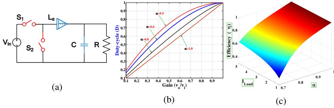
Fig. 8. (a) Buck converter. (b) Gain vs duty cycle. (c) The efficiency.
