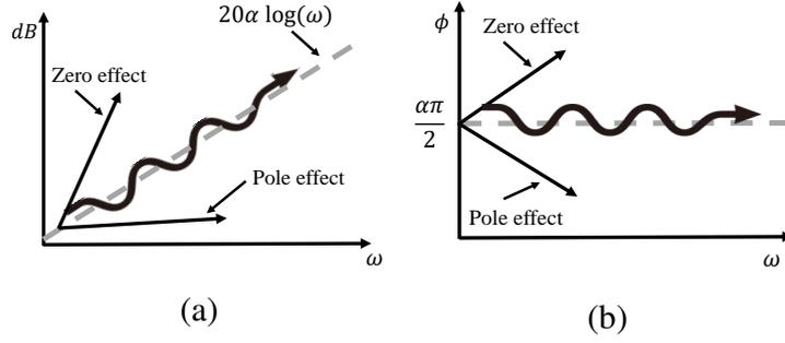
Fig. 2. Bode diagrams of  $s^\alpha$  (a) Magnitude of  $s^\alpha$  for any  $\alpha$  and (b) Phase of  $s^\alpha$  for any  $\alpha$ . are calculated for a given transfer function  $H(j\omega)$  as follows:
