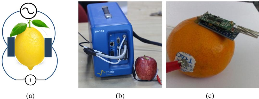
Fig. 7. (a) Bio-impedance measurement schematic. (b) SP150 impedance analyzer experimental setup. (c) Portable impedance analyzer.
