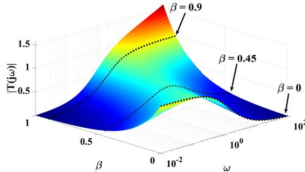
Fig. 6. Example of fractional-order simple fractional BPF.
