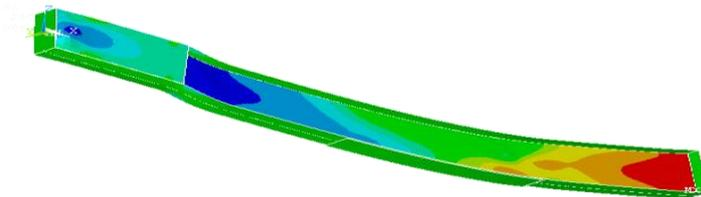
Fig. 13. Ultimate shear stresses (III, 6, 0.8, V8, H10, S3)
