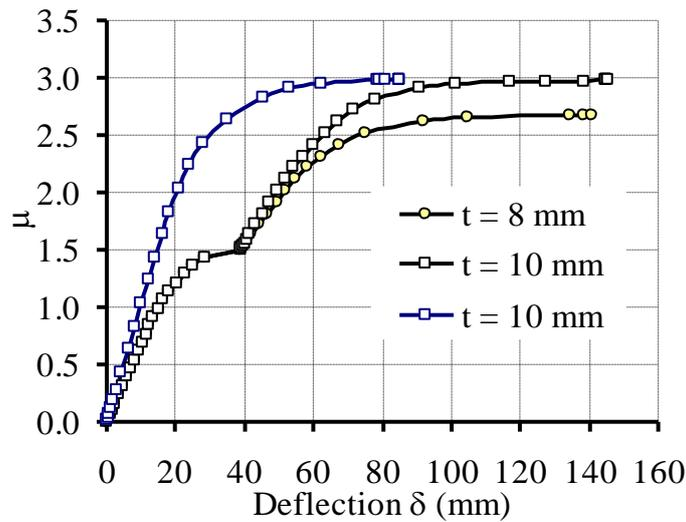
Fig. 5. Ultimate load demonstration of a strengthened beam (II, 8, 0.95, V\*).
