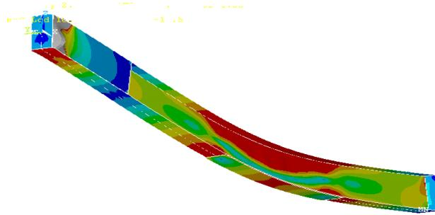
Fig. 11. The yield spread due strengthening plates at ULT2.
