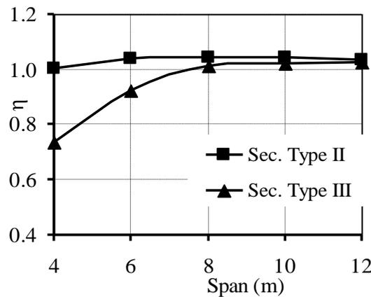
Fig. 4. The ultimate load of the un-strengthened proposed beams (ULT1).
