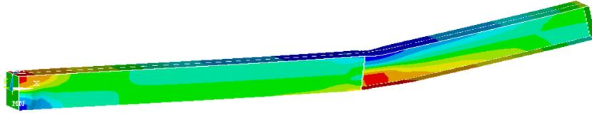
Fig. 7. Ultimate normal stresses (III, 6, 0.8, V8).
