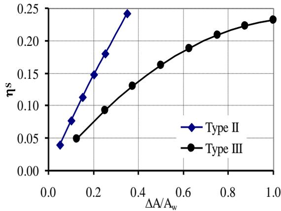
Fig. 10. Plastic moment increase due to horizontal plate.
