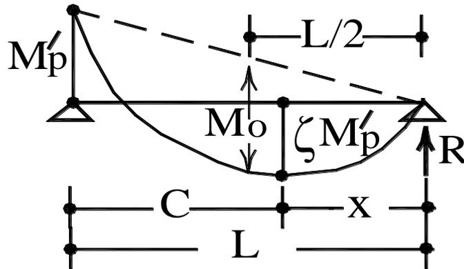
Fig. 3. Ultimate moment diagram of the strengthened beam.
