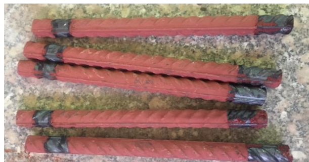
Fig. 3. Steel bars with epoxy zinc primer and uncoated spots.
