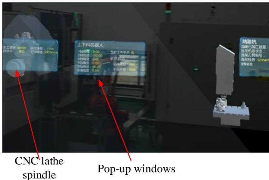
Fig. 12. Augmented reality display effect.
