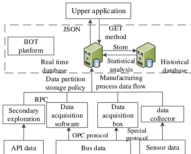
Fig. 5. Data collection process based on the industrial Internet of Things platform.
