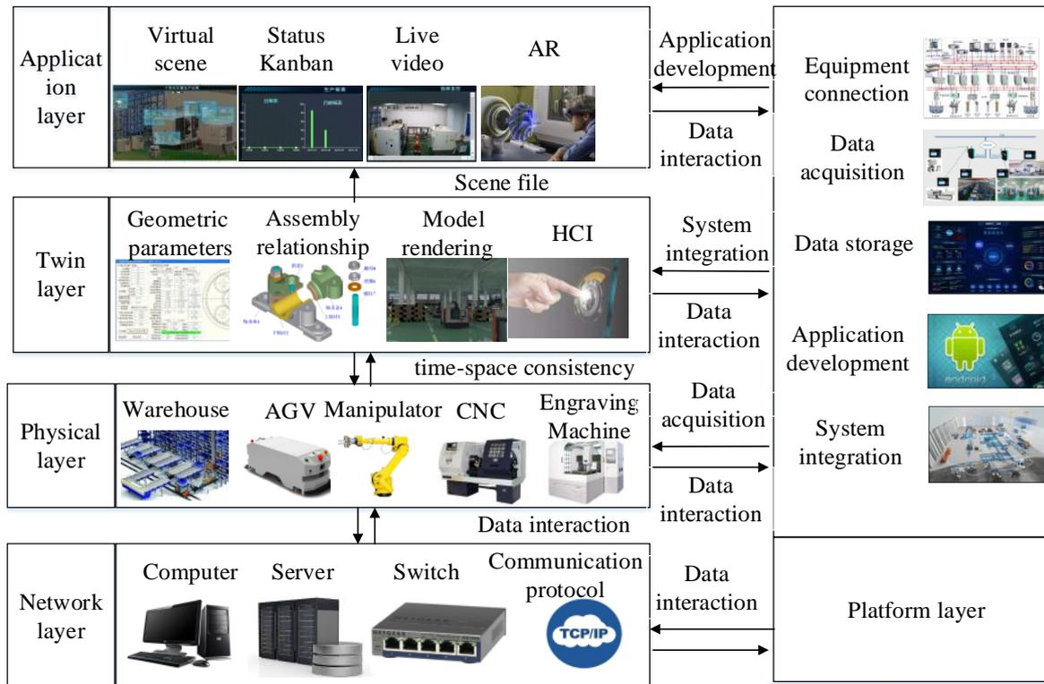
Fig. 1. Overall architecture of workshop 3D virtual monitoring system.
