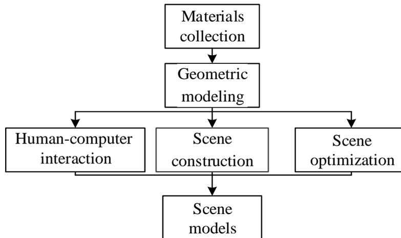
Fig. 3. Workshop virtual scene construction process.
