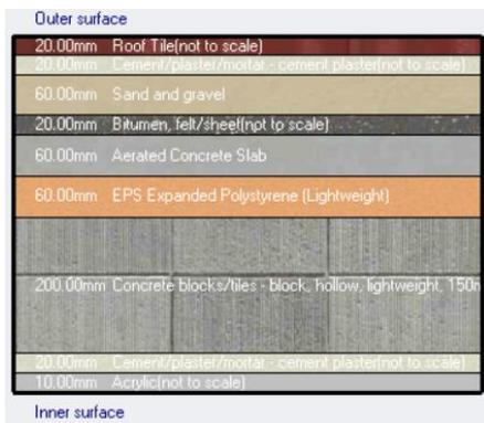
Fig. 10. Roof layers according to environmental code.
