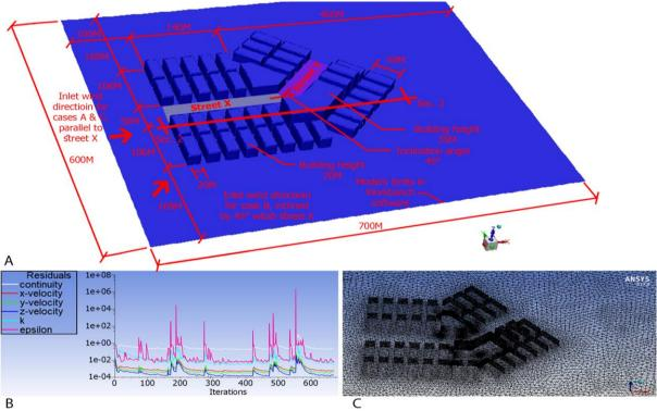
Fig. 4 Alternative 2, A) dimensions and inlet wind directions, B) Residuals by ANSYS Fluent software, C) Mesh by ANSYSWB module software.
