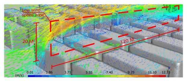
Fig. 9. Low wind speed zone created above buildings in alternatives 1 and 2 by ANSYS Fluent software (version19), inlet wind velocity 7m/s.
