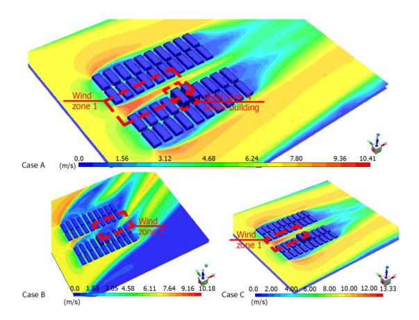
Fig. 5. Alternative 1, wind speed magnitude at height 15 m above street level in ANSYS Fluent software (version19) showing wind zones 1, 2 and 4.
