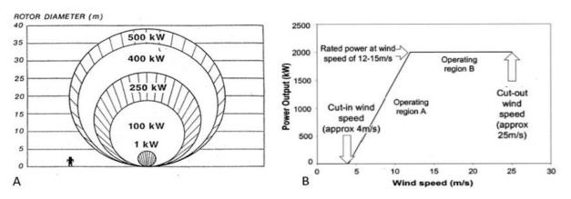
Fig. 2. A) Rotor diameter versus output generated power, B) Wind speed versus generated power output, [21].
