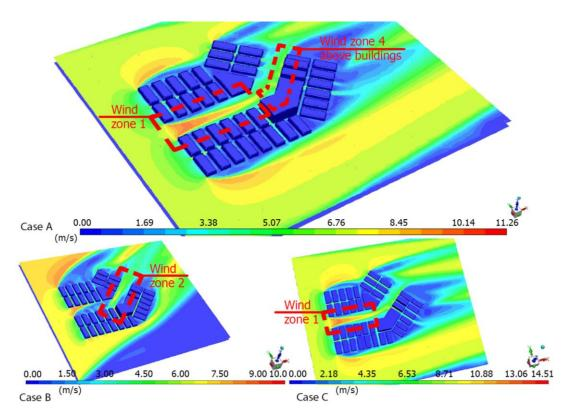
Fig. 6. Alternative 2, wind speed magnitude at height 15 m above street level in ANSYS Fluent software (version19) showing wind zones 1, 2 and 4.
