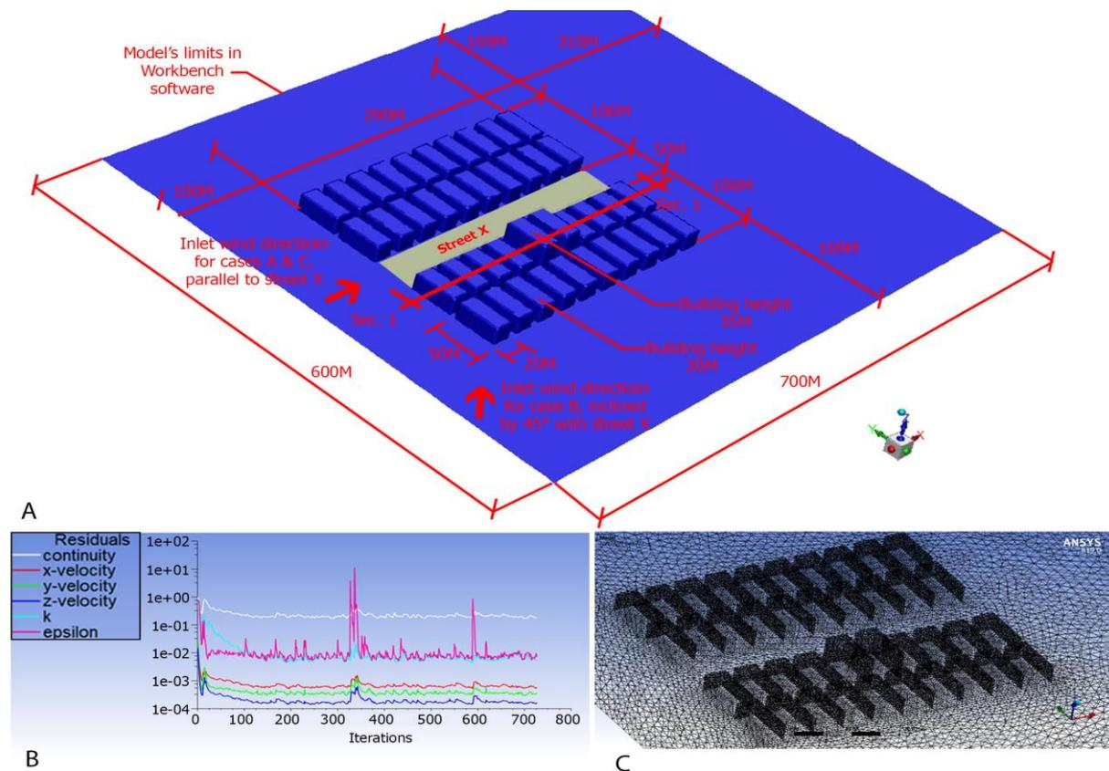
Fig. 3 Alternative 1, A) dimensions and inlet wind directions, B) Residuals by ANSYS Fluent software, C) Mesh by ANSYSWB module software.
