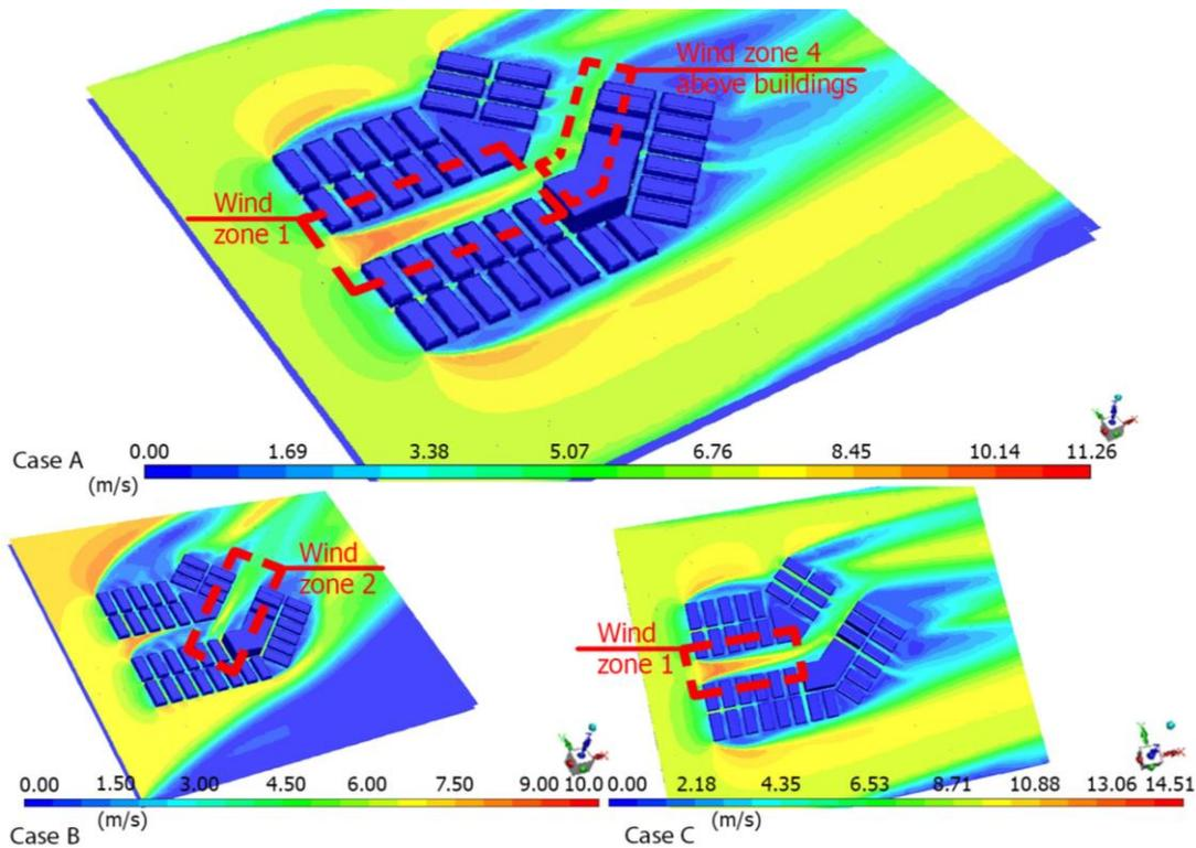
Fig. 6. Alternative 2, wind speed magnitude at height 15 m above street level in ANSYS Fluent software (version19) showing wind zones 1, 2 and 4.
