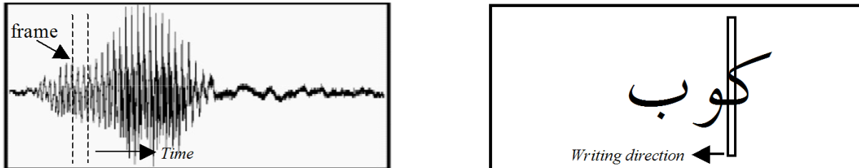
Fig. 6. Sliding window over a speech signal and over a text image bitmap.
